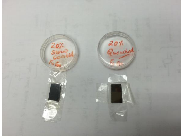
Figure E.1: Galfenol single crystal samples 20 at. % Ga composition that were oven cooled and quenched used in kerr microscopy.
